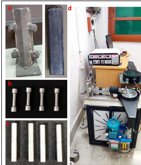
Fig. 1. (a) Mold and ascast sample, (b) Tensile samples, (c) Pin sample for wear and friction test, (d) Pin-on-disc tribometer
