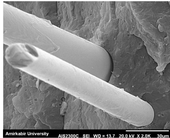
Fig. 5. SEM micrograph of the composite specimen containing 1 wt% graphene nanoparticles, 20 wt% basalt fibers, and 30 wt% SMR20
