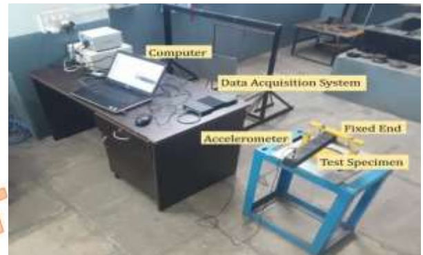
Fig. 9. Actual photograph of Vibration damping measuring tests
