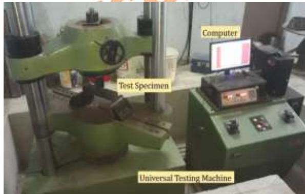
Fig. 7. Actual photograph of Three-point flexural test
