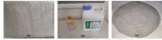
Fig. 1. Raw materials used in the development of the composite: (a) Kenaf mat; (b) Epoxy matrix; and (c) Cenosphere.
