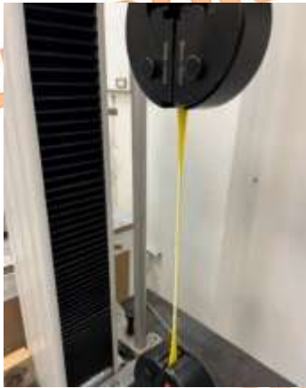
Fig. 10. Tensile testing of the standard specimens
