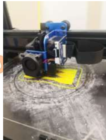
Fig. 6. 3D-printed standard specimens for tensile testing
