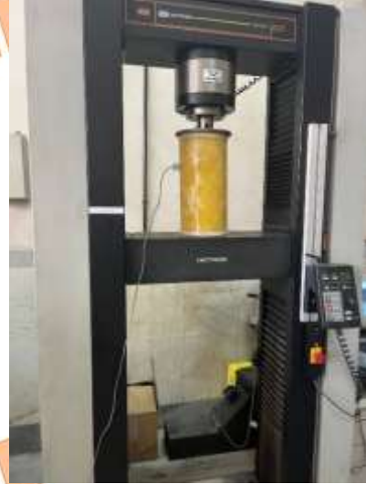
Fig. 11. Modal test setup of the experimental specimens
