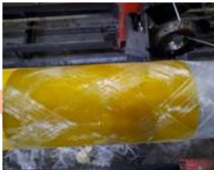
Fig. 7. Fiber winding process
