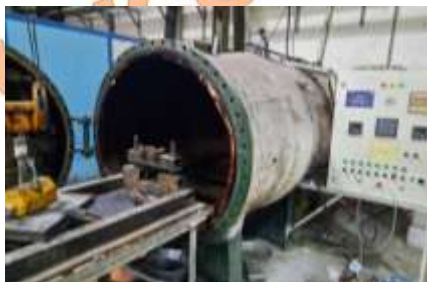
Fig. 8. Final curing process of the specimens
