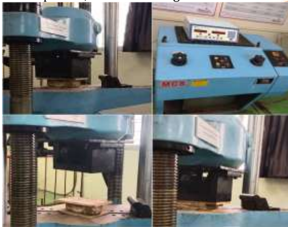
Fig. 9: Compression test (UTM)
