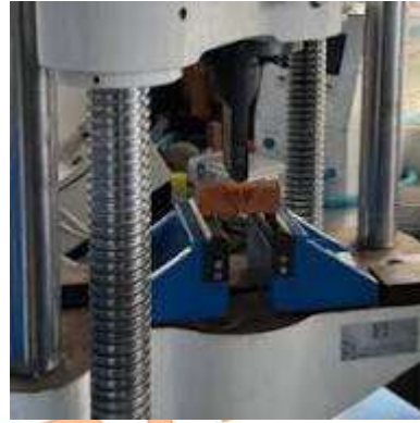
Fig. 10: Three-point bending flexural testing
