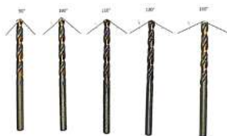
Fig. 6. 5 mm Diameter Drill Bits with Varying Point Angles
