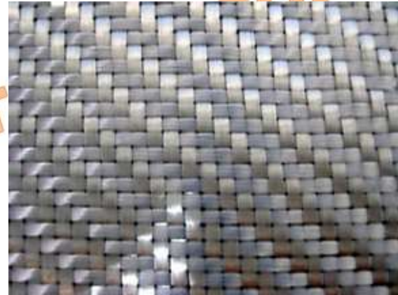
Fig. 1. Satin Weave Pattern of E-Glass Fabric Used in Composite Specimen Fabrication
