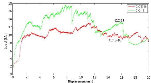
**Figure 14.** Load-displacement curves of specimens with the same geometrical characteristics and different filling conditions
