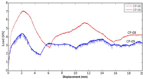
**Figure 7.** Comparison of load-displacement diagrams of empty copper tubes with different diameters
