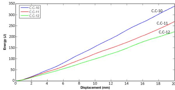
**Figure 10.** Comparison of energy–displacement diagrams of copper tubes reinforced by carbon/epoxy composite tubes with different diameters
