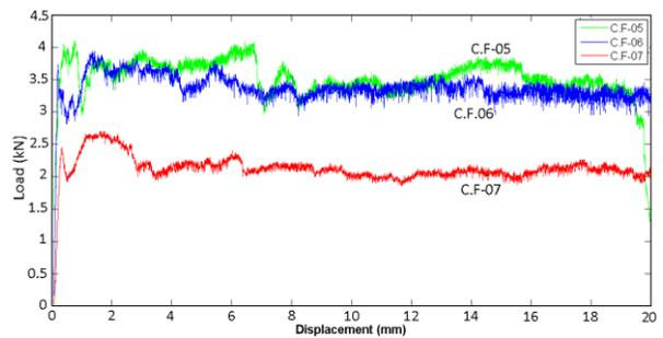
**Figure 4.** Comparison of load-displacement diagrams of silicone sealant-filled carbon/epoxy composite tubes with different diameters
