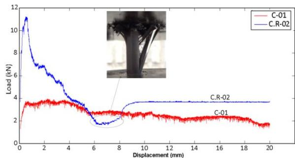
**Figure 5.** Comparison of load-displacement diagrams of an empty carbon/epoxy composite tube and a carbon/epoxy composite rod
