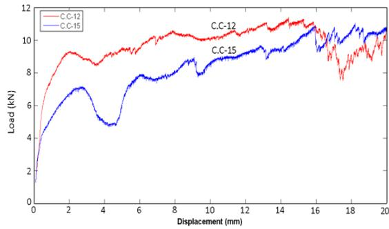
**Figure 11.** Comparison of load–displacement diagrams of copper tubes with different diameters reinforced by carbon/epoxy composite tubes with the same diameter
