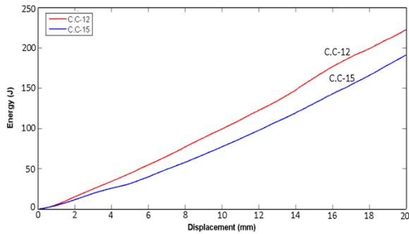
**Figure 12.** Comparison of energy–displacement diagrams of copper tubes with different diameters reinforced by carbon/epoxy composite tubes with the same diameter
