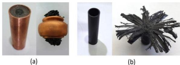
**Figure 1.** (a) The specimen C.C-15 before and after axial test, (b) The specimen C-01 before and after axial test
