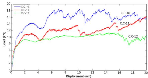
**Figure 9.** Comparison of load-displacement diagrams of copper tubes reinforced by carbon/epoxy composite tubes with different diameters
