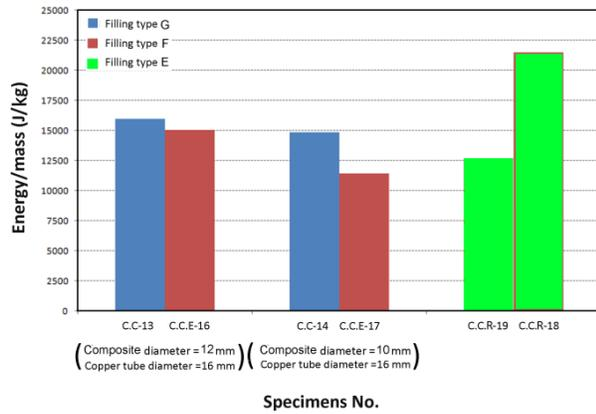
**Figure 15.** SAE of copper tubes reinforced with carbon/epoxy composite tubes by different filling conditions
