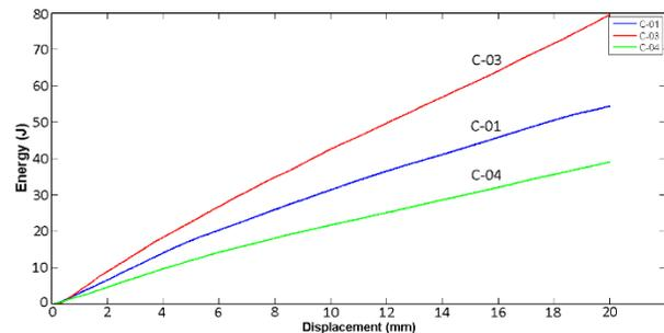
**Figure 3.** Comparison of energy–displacement diagrams of empty carbon/epoxy composite tubes with different diameters
