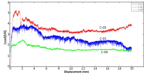
**Figure 2.** Comparison of load–displacement diagrams of empty carbon/epoxy composite tubes with different diameters
