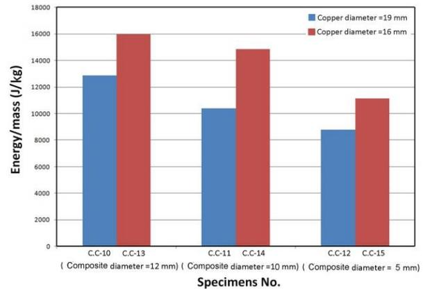
**Figure 13.** Comparison of SAE of reinforced copper tubes with carbon/epoxy composite tubes (type G in Table 2)
