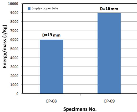
**Figure 8.** Comparison of SAE by the empty copper tubes with different diameters
