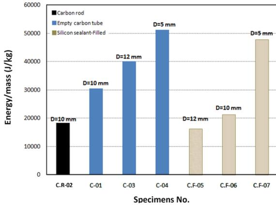
**Figure 6.** Comparison of SAE of empty and silicon sealant-filled carbon/epoxy composite tubes and also, carbon/epoxy composite rod
