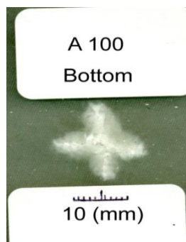
Figure 4. Damage in the impacted bottom layer of A100
