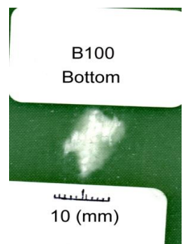
Figure 5. Damage in the impacted bottom layer of B100
