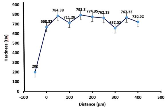
Fig. 6. Microhardness profiles for HVOF sprayed NiCrBSi coatings on the carbon steel
