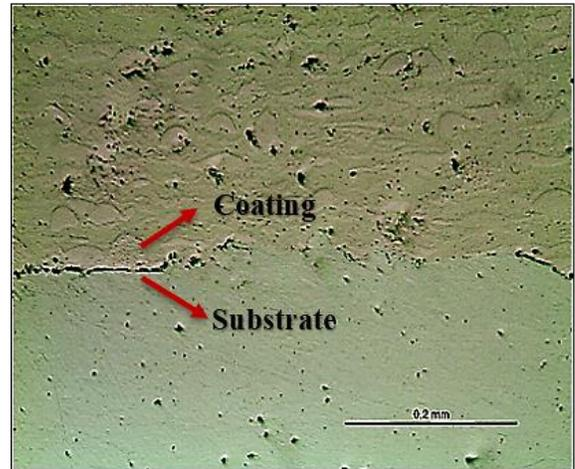
Fig. 2. Optical micrographs of polished cross sections
