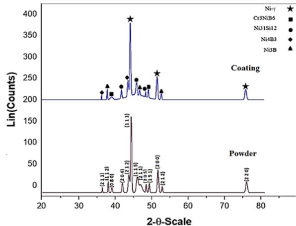
Fig. 5. XRD patterns of the feedstock powder and as-sprayed coating.
