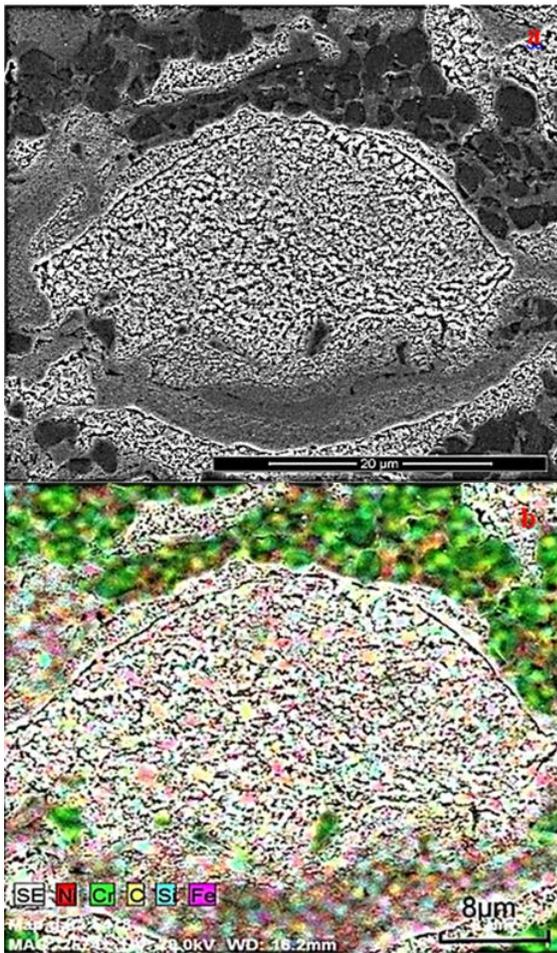
Fig. 4. SEM images showing (a) the morphology of the coating and (b) the corresponding map spectra
