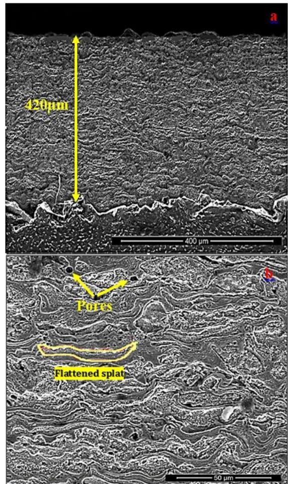
Fig. 3. SEM images of a transverse section of the as-sprayed coating: (a) a lamellar morphology; and (b) pores
