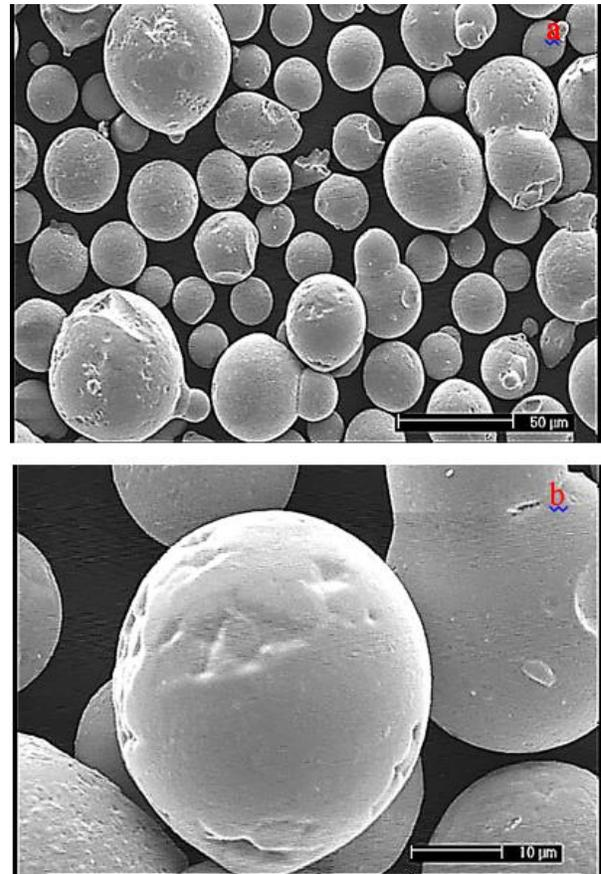
**Fig. 1.** SEM micrographs of the powder morphology at a magnification of (a) 500x and (b) 2000x.
