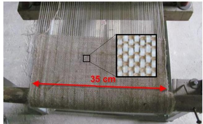
Fig. 4. The weaver machine weaving the hybrid tissue with the pattern
