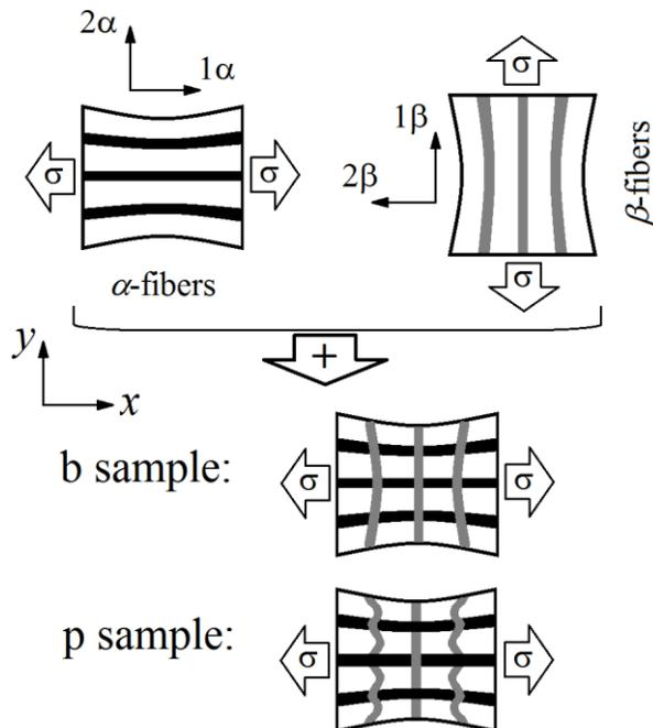
Fig. 14. The effect of fibers posture on matrix reinforcement
