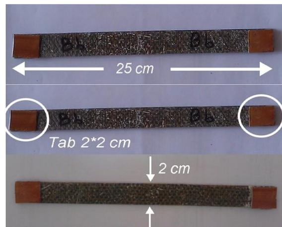
Fig. 6. The appearance and dimensions of some specimens
