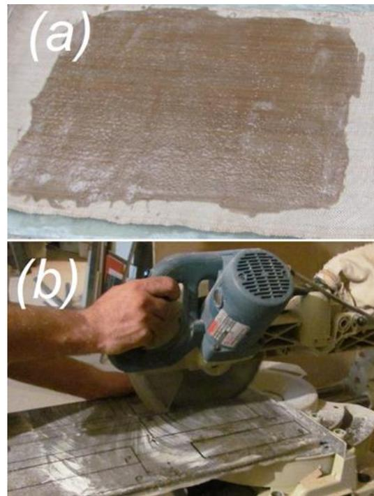
Fig. 5. Preparation of tensile test specimens a) coating tissue with resin b) cutting the composite plates
