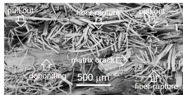
**Fig. 13.** The SEM micrograph of the broken composite surface
