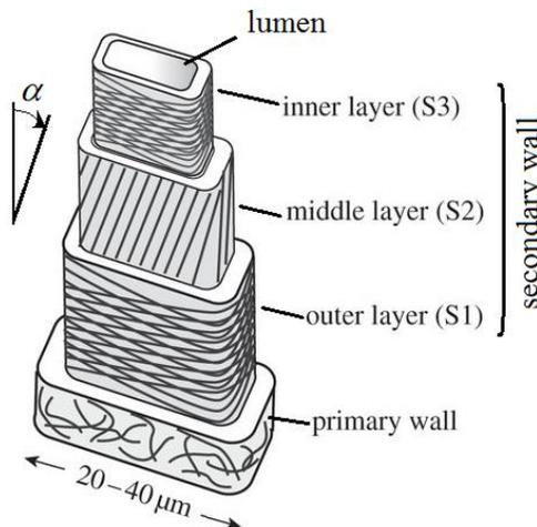
Fig. 1. Constituent layers of a hemp fiber
