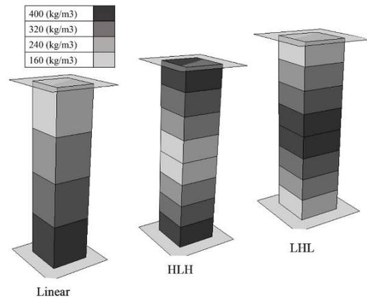
**Fig. 3.** Schematic of layered foam-filled specimens with different densities.
