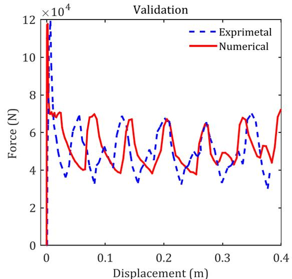
**Fig. 4.** Comparison of experimental Force- Displacement curves with numerical results [5].
