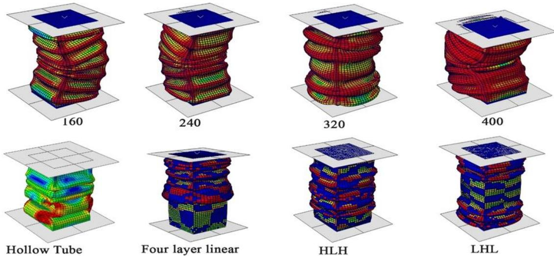
Fig. 5. Final deformed shape of specimens
