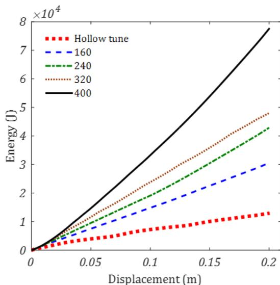
Fig. 6. Energy- displacement curves of uniform density foam-filled specimens compared to the empty tube.
