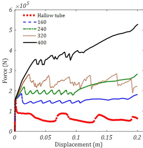
Fig. 8. Load- displacement Curves of Uniform Foam-filled specimens compared to the empty tube.
