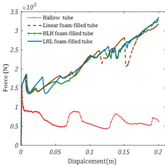
Fig. 9. Load- displacement Curves of Uniform Foam-filled specimens compared to the empty tube.
