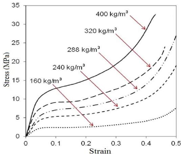
Fig. 1. Experimental true stress-strain curves for foam specimens with various nominal densities [16].
