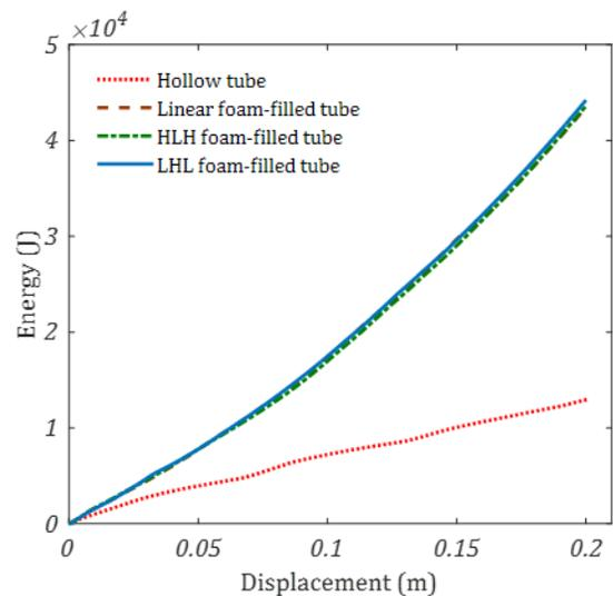
Fig. 7. Energy- displacement Curves of layered Foam-filled specimens compared to the empty tube.
