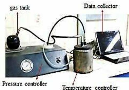
Fig. 7. Designed apparatus for pressure failure testing.
