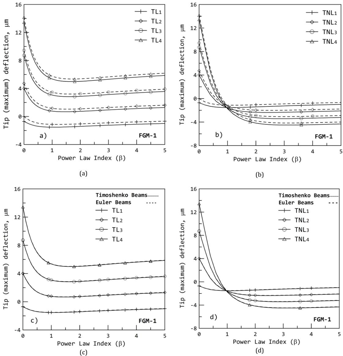
Fig. 8. Effect of shear deformation on variation in maximum (tip) deflection with ( $\beta$ )- a) LTD; b) NLTD; c) LTD; d) NLTD
