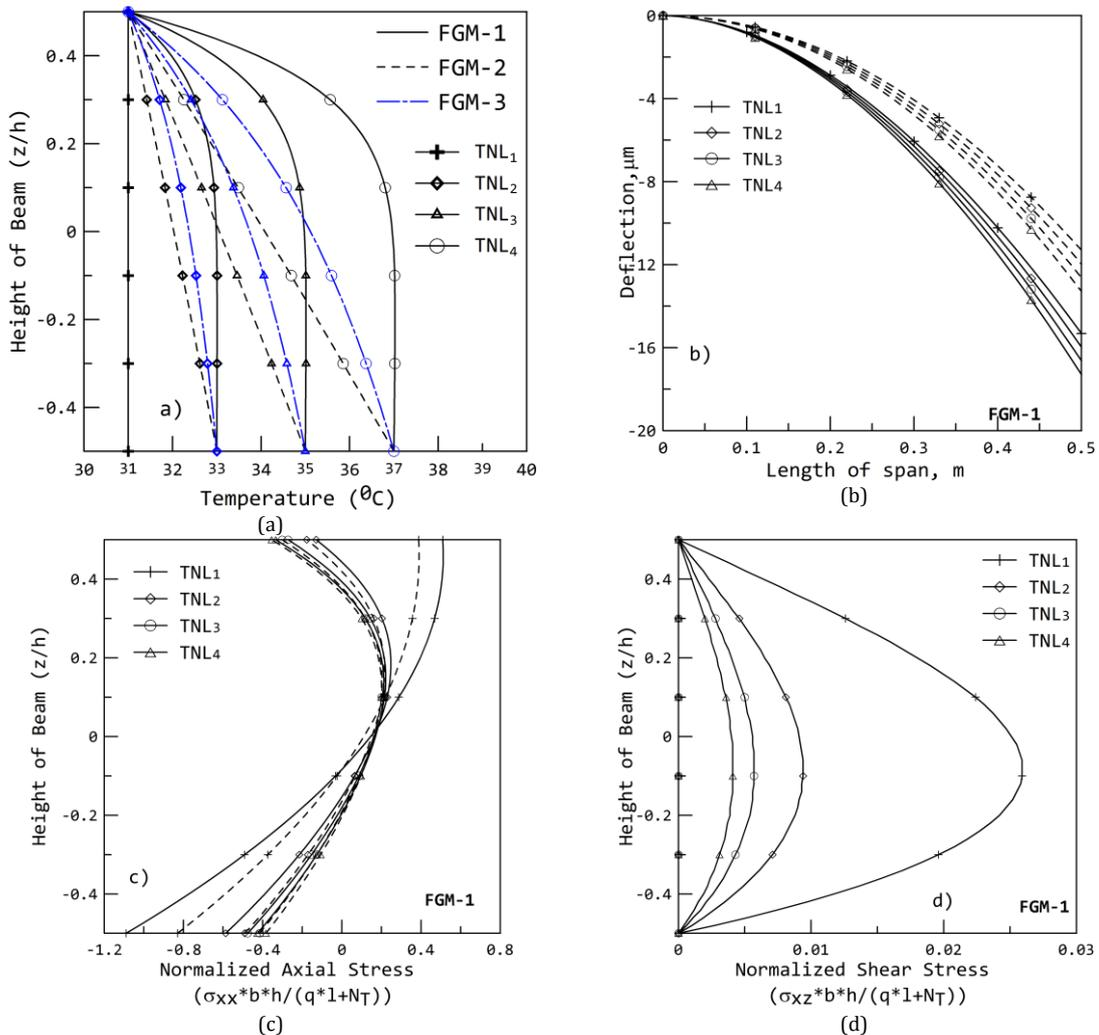
**Fig. 7.** For  $\beta=1$  & Nonlinear temperature distribution, a) Distribution of temperature across the beam height; b) Transverse Deflection; c) Normalized Axial stresses at the fixed end; d) Normalized Shear stresses at fixed end
