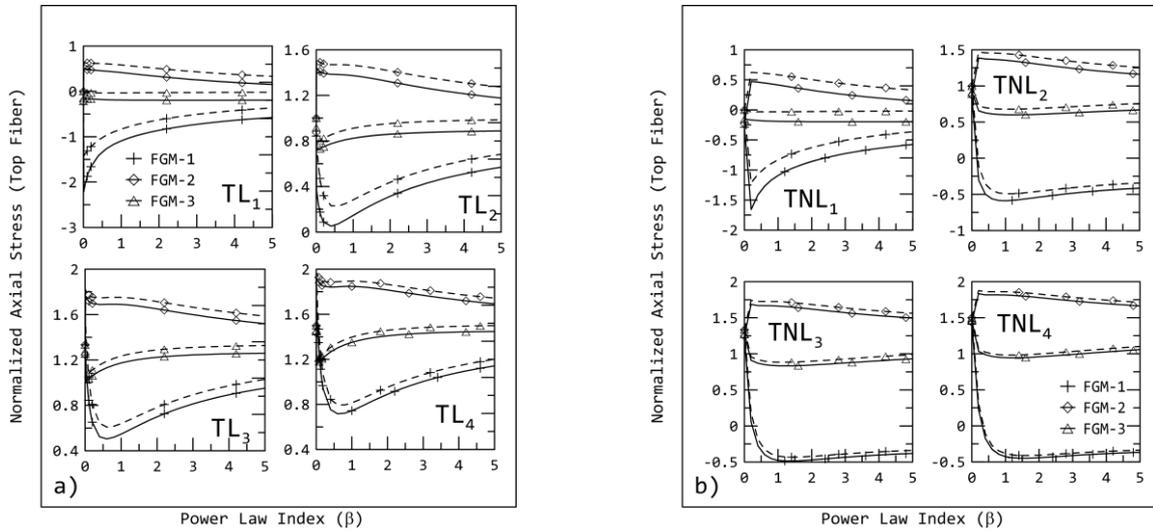
Fig. 16. Variation in normalized axial stress of FGM-1 with Power law index ( $\beta$ ) a) Linear Distribution, TL3; b) Nonlinear Distribution, TNL3
