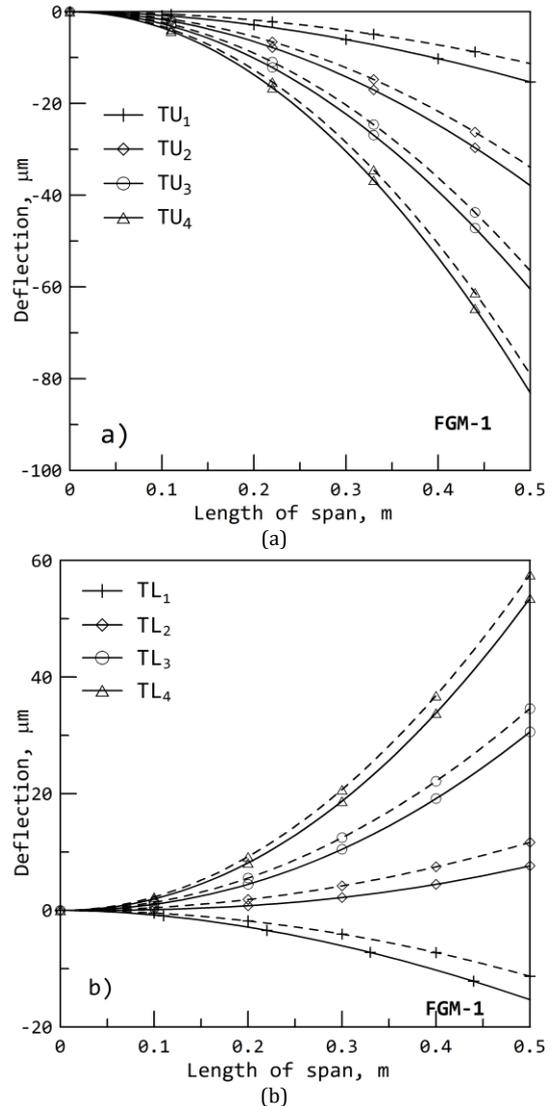
Fig. 4. Transverse Deflection of C-F beam (FGM-1) for  $\beta=1$  a) Uniform temperature; b) Linear Temperature Distribution
