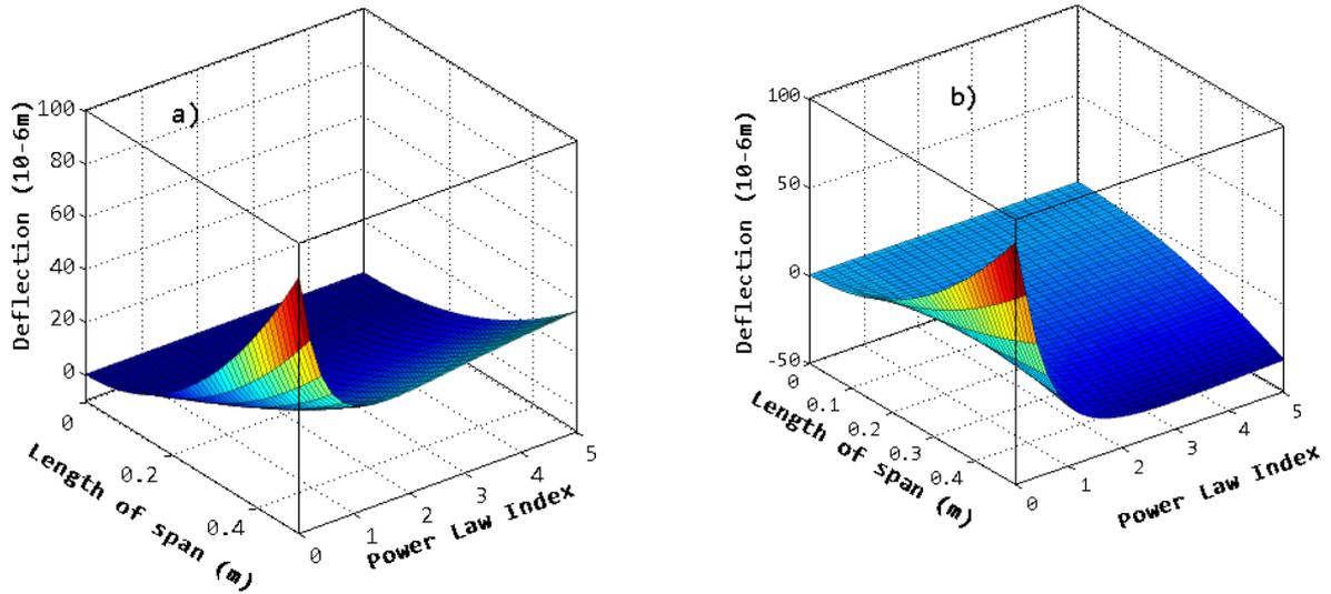
Fig. 12. Variation in transverse deflection of FGM-1 with Power law index ( $\beta$ ) a) Linear Distribution, TL3; b) Nonlinear Distribution, TNL3
