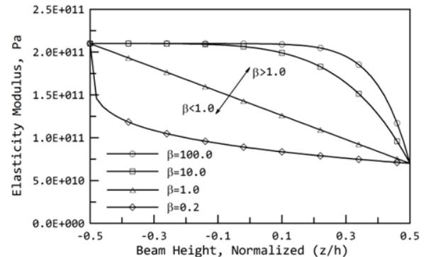
Fig. 2. Variation of Modulus of Elasticity across the cross-section with power law index, β
