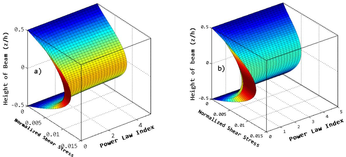
Fig. 14. Variation in normalized shear stress of FGM-1 with Power law index ( $\beta$ ) a) Linear Distribution, TL3; b) Nonlinear Distribution, TNL3
