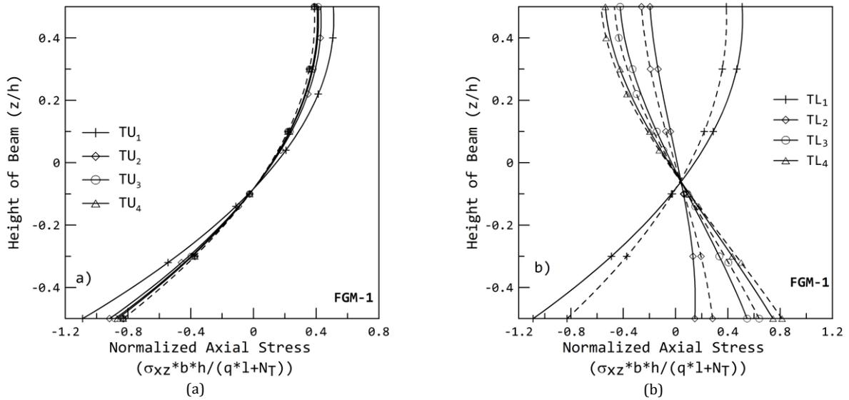
Fig. 5. Axial Stresses (Normalized) at the fixed end of the C-F beam (FGM-1) for  $\beta=1$  a) Uniform Temperature; b) Linear Temperature Distribution
