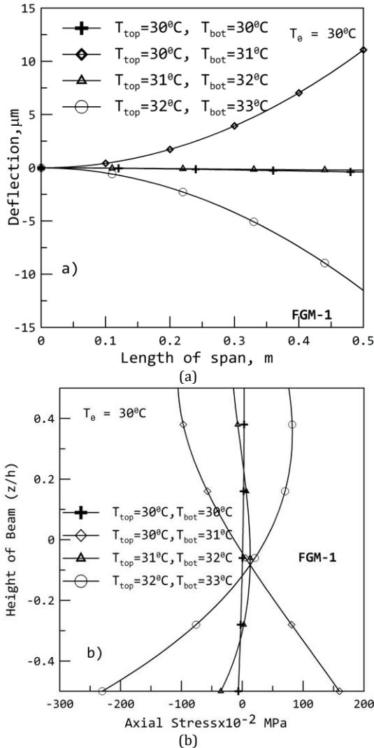
Fig. 3. a) Transverse Deflection b) Normalized Axial Stress (at the fixed end) of C-F beam (FGM-1) for  $\beta=1$
