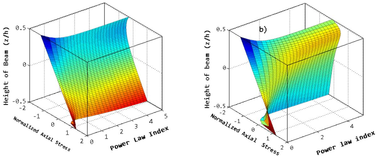
Fig. 13. Variation in normalized axial stress of FGM-1 with Power law index ( $\beta$ ) a) Linear Distribution, TL3; b) Nonlinear Distribution, TNL3
