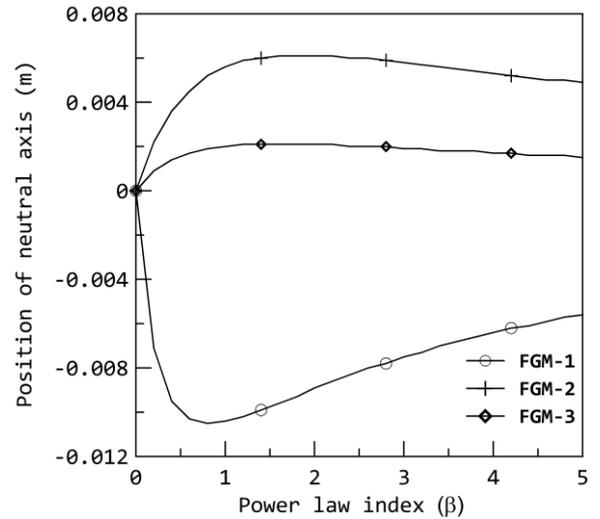
Fig. 9. Variation in the position of neutral axis with ( $\beta$ )
