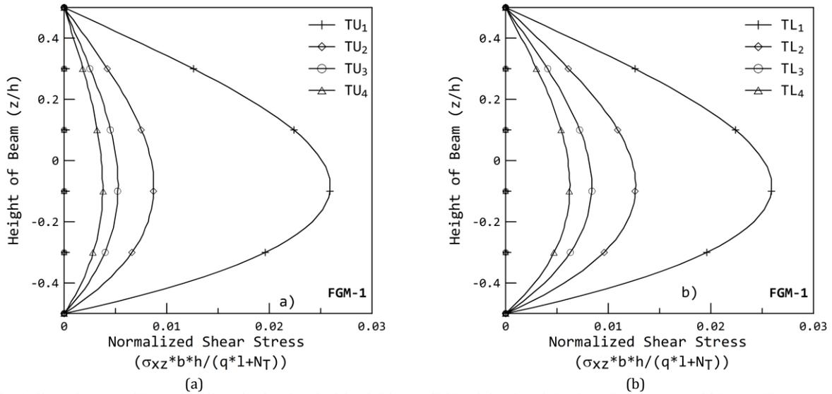
Fig. 6. Shear Stresses (Normalized) at the fixed end of the C-F beam (FGM-1) for  $\beta=1$  a) Uniform Temperature; b) Linear Temperature Distribution
