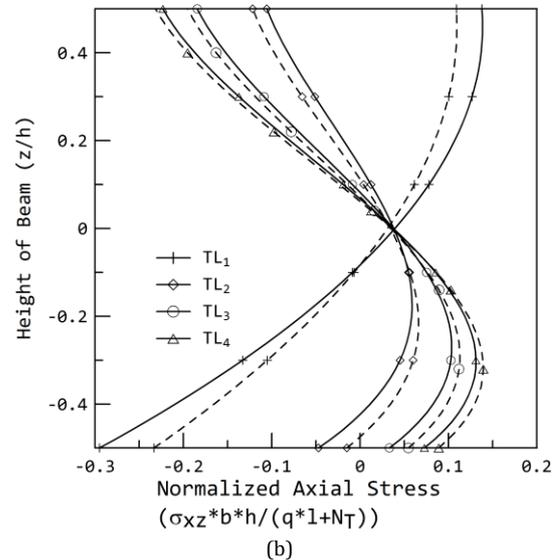
Fig. 10. C-S beam under the thermal and thermo-mechanical load of (FGM-1) for  $\beta=1$  a) Transverse Deflection; b) Normalized Axial Stress
