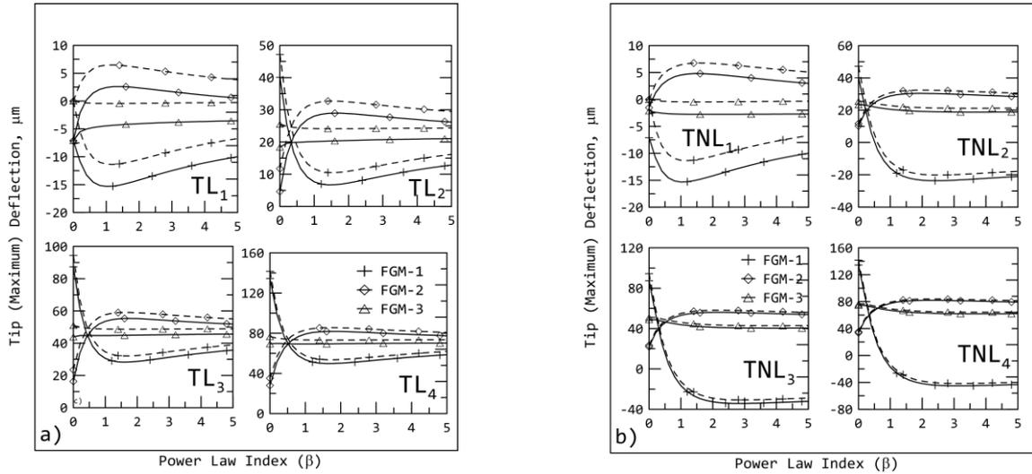
Fig. 15. Variation in transverse deflection of FGM-1 with Power law index ( $\beta$ ) a) Linear Distribution, TL3; b) Nonlinear Distribution, TNL3
