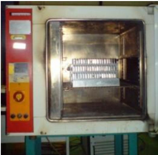
Figure 1. The front view of the composite specimens in the designed aluminum container inside the oven.
