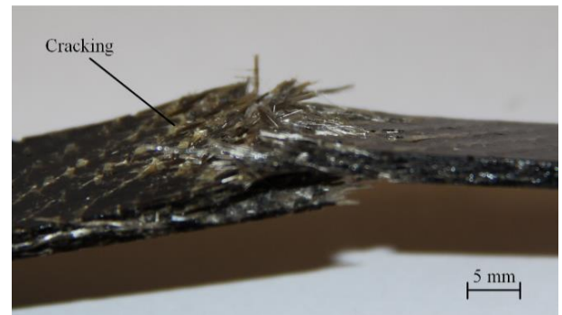
Figure 8. The fractured specimen of WBP composite exposed to the accelerated heat ageing at 150 °C after the tensile test.
