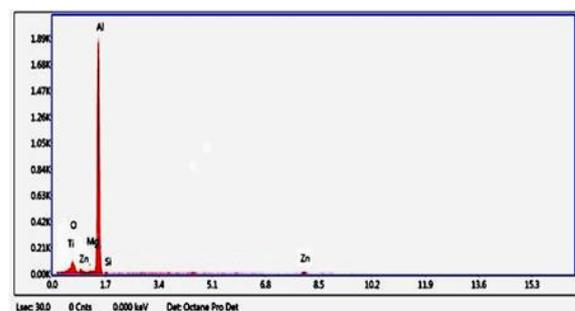
Fig. 6. Showing the energy dispersive spectrum analysis of Al7075-10wt. % nano TiO<sub>2</sub> composite
