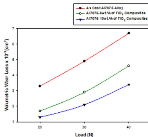
Fig. 12. Volumetric wear loss of Al7075 alloy and nano TiO<sub>2</sub> composites at varying loads and 400 rpm constant speed
