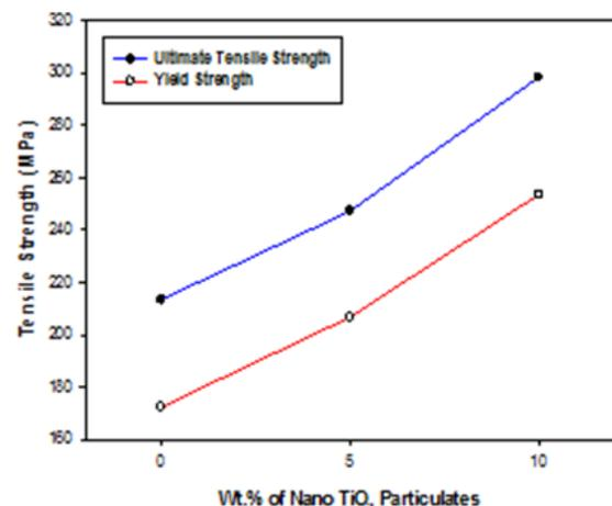
Fig. 9. Ultimate tensile and yield strength of Al7075 alloy and nano TiO<sub>2</sub> composites
