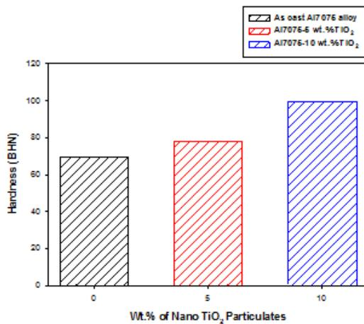
Fig. 8. The hardness of Al7075 alloy and nano TiO<sub>2</sub> composites
