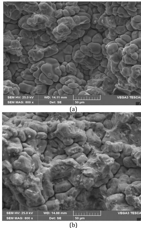
Fig. 11. Fracture surfaces of samples tested for the tensile test (a) Al7075 matrix alloy (b) Al7075-10wt. % nano TiO<sub>2</sub> composite
