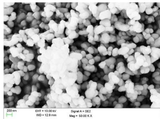
**Fig. 1.** SEM photograph of nano TiO<sub>2</sub> Particles used in the study
