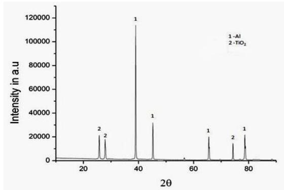
Fig. 7. Showing XRD analysis of Al7075 alloy with 10wt. % nano TiO<sub>2</sub> composite
