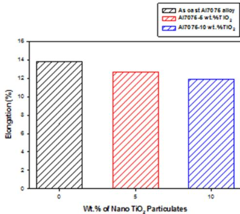
Fig. 10. Percentage elongation of Al7075 alloy and nano TiO<sub>2</sub> composites
