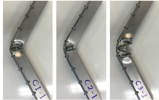
Fig. 14. Folding pattern in experimental tests.
