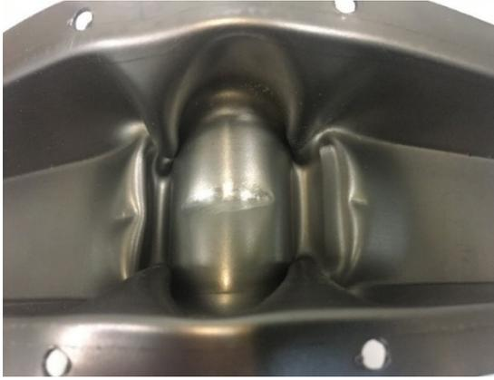
Fig. 15. Top-hat of specimen C3 from inside.
