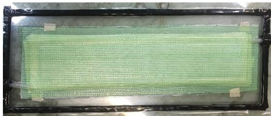
Fig. 4. Vacuum assisted resin transfer molding.
