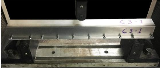
Fig. 1. Experimental setup for the quasi-static three-point bending tests.
