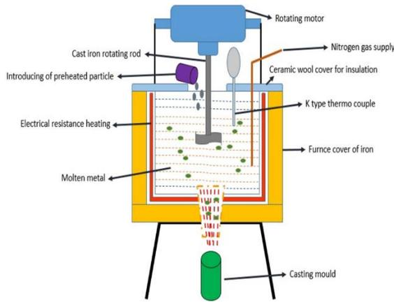
Fig. 1. The schematic of the stir casting furnace
