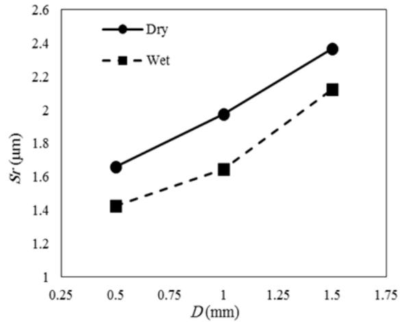
**Fig. 11.** The Effect of depth of cut on surface roughness
