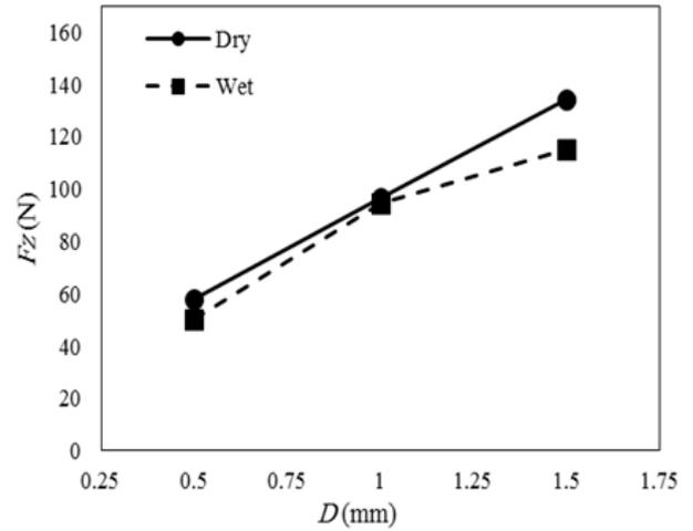
Fig. 7. The effect of depth of cut on the cutting force
