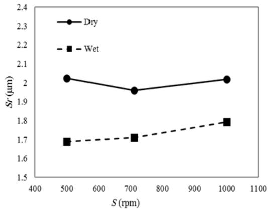
**Fig. 9.** The Effect of spindle speed on surface roughness
