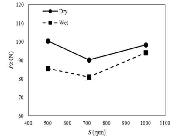
**Fig. 5.** The effect of spindle speed on the cutting force
