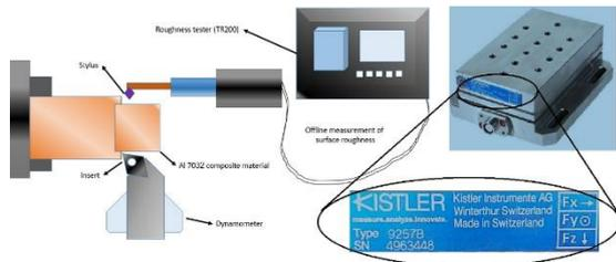
Fig. 3. the schematic of the machining setup
