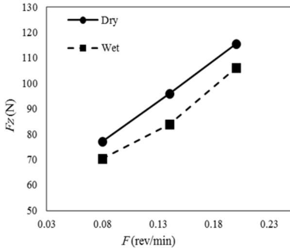
Fig. 6. The Effect of feed rate on the cutting force
