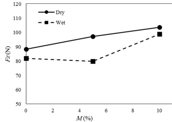
**Fig. 4.** the effect of reinforcement's percentage on the cutting force
