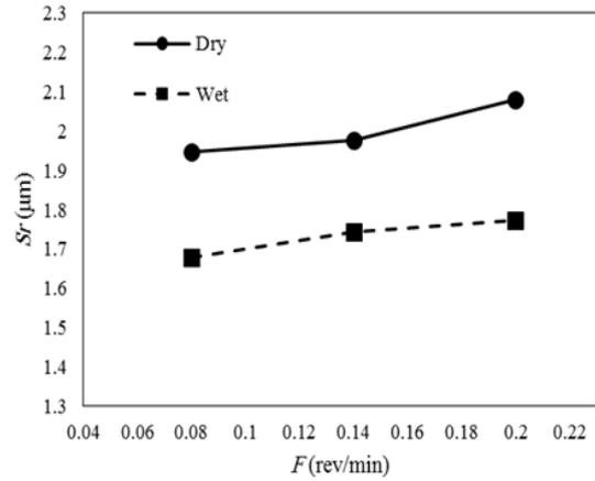
**Fig. 10.** The Effect of feed rate on surface roughness
