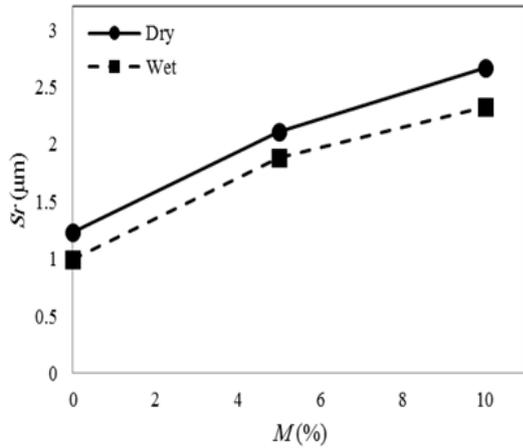
**Fig. 8.** The Effect of reinforcements percentage on surface roughness
