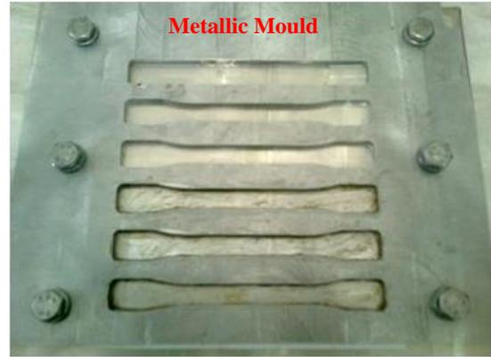
Fig. 2. The fabricated metallic mould
