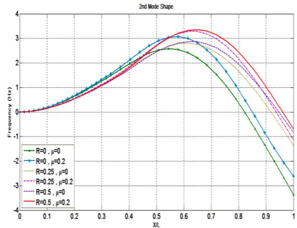
Fig. 3. The second mode shape of the nanobeam for different sensed mass
