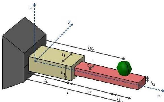
Fig. 1. Nonlocal mass sensor cantilever nanobeam
