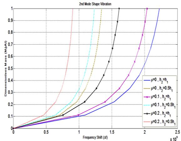
**Fig. 5.** The shift of the second natural frequency of the mass sensor nanobeam
