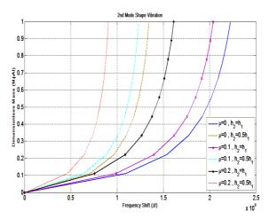
**Fig. 5.** The shift of the second natural frequency of the mass sensor nanobeam
