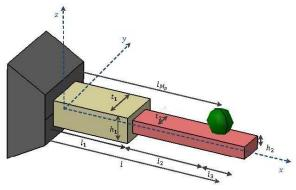
Fig. 1. Nonlocal mass sensor cantilever nanobeam
