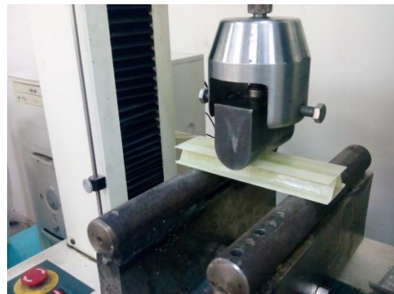
Fig. 14. HOUNSFIELD machine used for three-point bending test.
