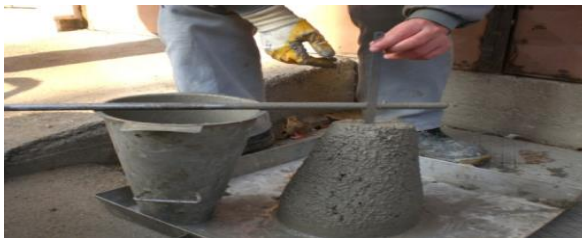
Fig. 3. Measuring the concrete slump
