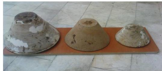
Fig. 1. wooden models used for making samples
