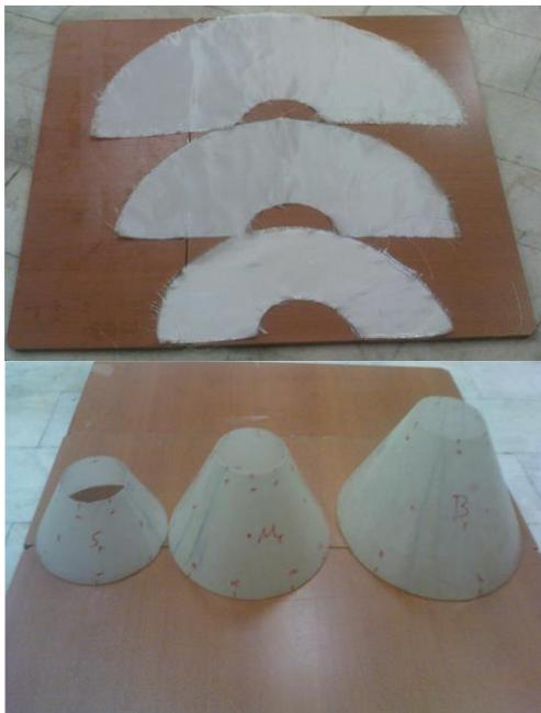
Fig. 3. above: cut cloths, down: composite samples
