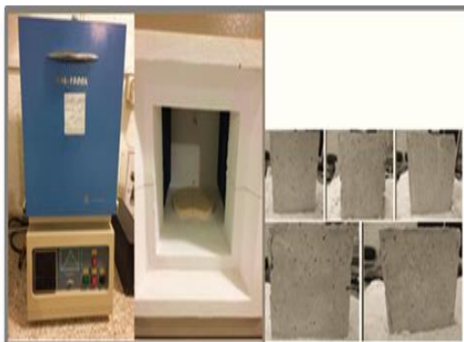
Fig 1. The oven used for heating the specimens
