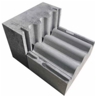
(b) Arc-shaped corrugated mold
