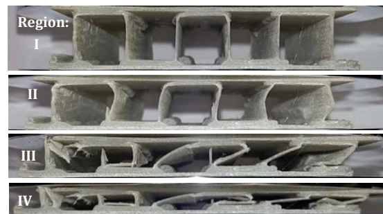
Fig. 7. Image of progressive damage development in rectangular corrugated core sandwich panel
