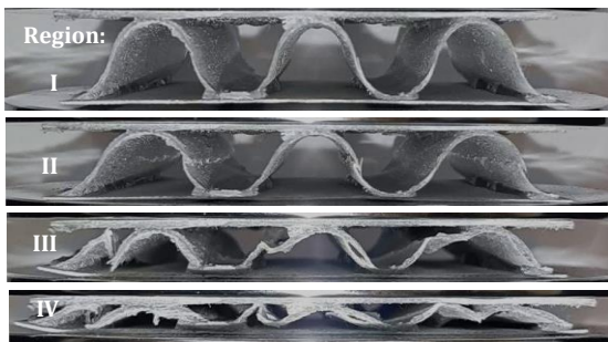
Fig. 15. Image of progressive damage development in arc-shaped corrugated core sandwich panel
