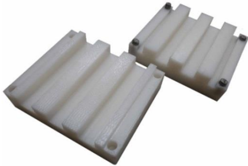
Fig. 2. Rectangular corrugated mold made of Teflon
