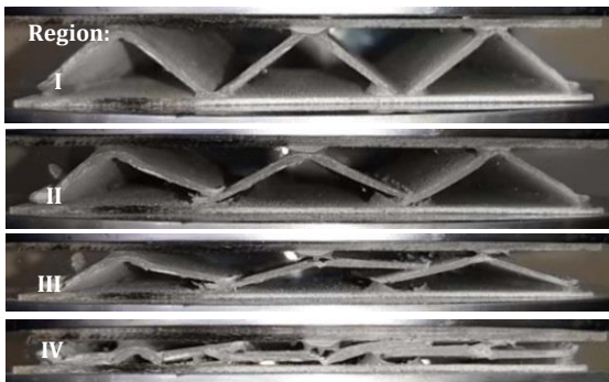
Fig. 11. Image of progressive damage development in triangular corrugated core sandwich panel
