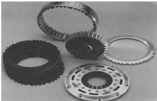
Fig.2. Carbon disk clutch system of a Formula1 racing car [1]
