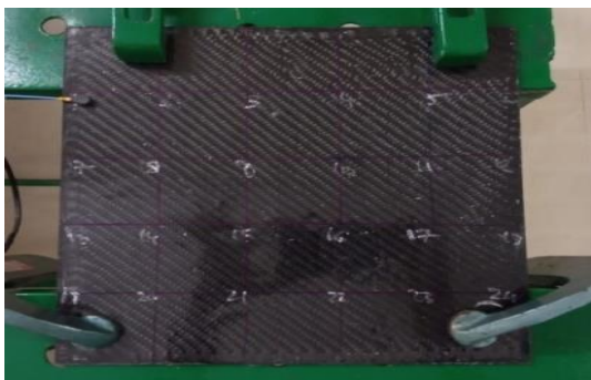
Fig. 9. Hybrid square plate with CFCF Boundary condition
