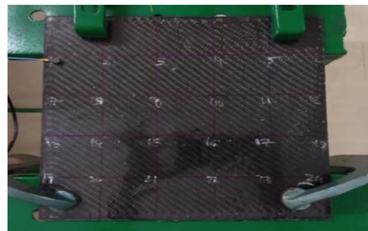
Fig. 4. CFRP square plate with CFCF Boundary condition
