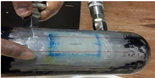
Fig. 6. Composite patch leakage under internal pressure
