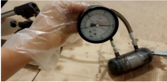
Fig. 5. Hydrostatic testing for the repaired steel pipe
