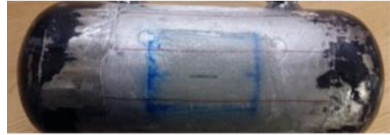
Fig. 3. Schematic of repaired steel pipes
