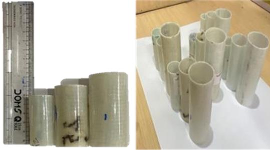
Fig. 3. Composite tubes with different inner diameters containing different extents of overlap
