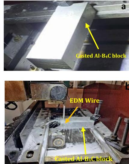
Fig. 3. (a) Machined sample of Al-B4C composite (b) W-EDM machine
