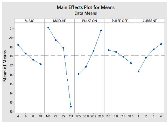
Fig. 6. Mean Effect plot for Surface roughness
