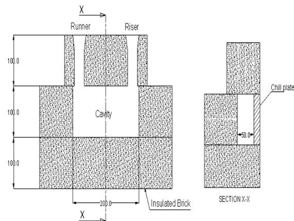
**Fig. 1.** Sectional front view and cross-sectional view of the mold [10].
