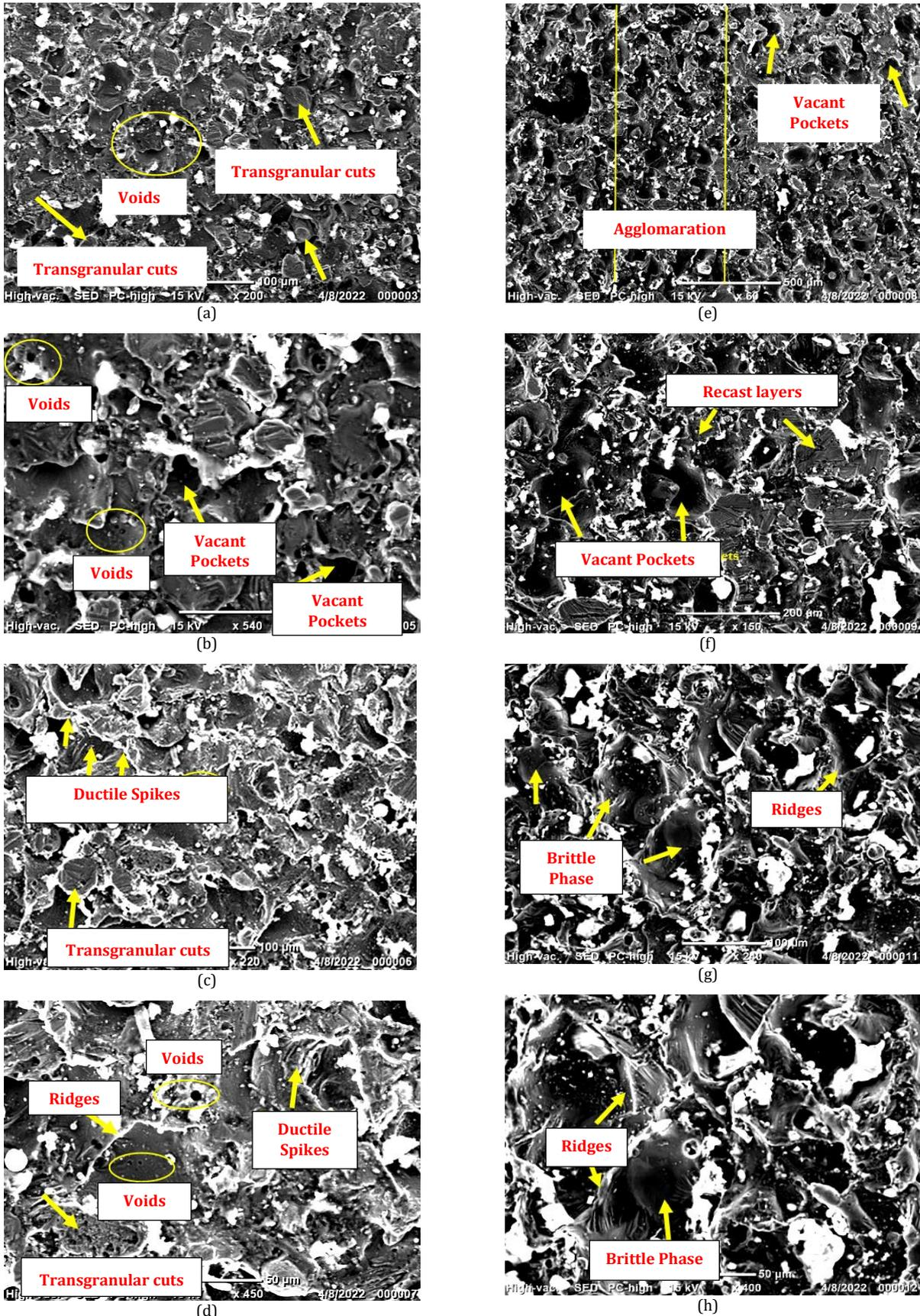
Fig. 7. SEM image of specimen (a-b) 4% B4C-MS chill (c-d) 6% B4C-CI chill (e-f) 8% B4C-SS chill (g-h) 10% B4C - Cu chill
