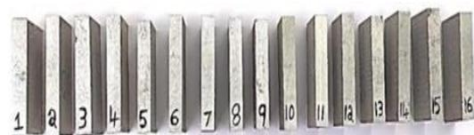
Fig. 4. Cut specimens from the composite series
