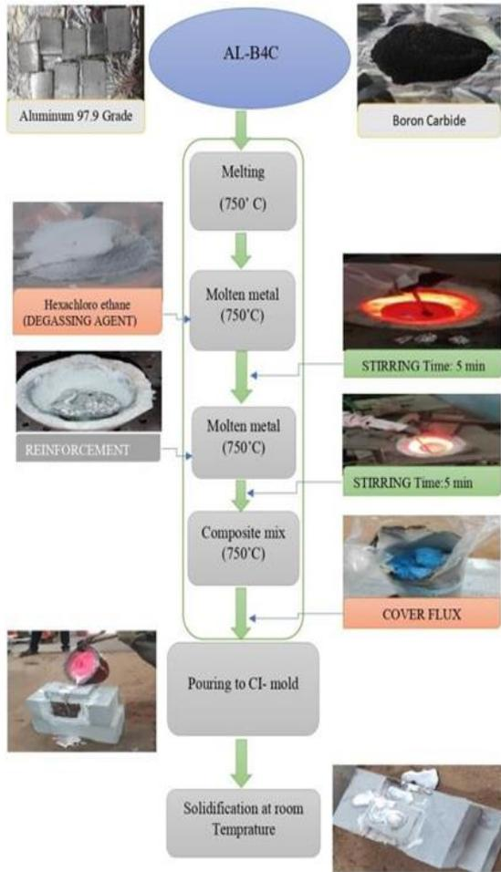
Fig. 2. Sequential procedure used in stir casting process
