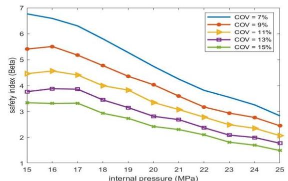
Fig. 8. Safety index in terms of the different COV of the ultimate strength
