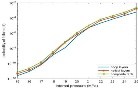
Fig. 3. Probability of failure of the composite tank in terms of internal pressure
