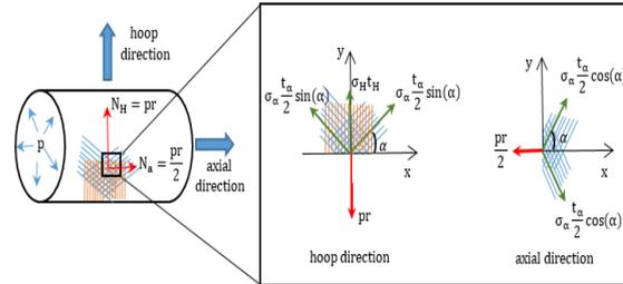
Fig. 1. Combinations of the hoop and helical layers in the hoop and axial directions
