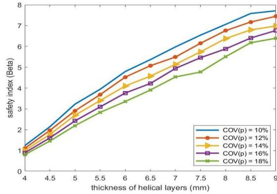
Fig. 16. Safety index of the helical layers of the composite tank in terms of helical thickness with the variation of different COV of the internal pressure (P=20MPa)
