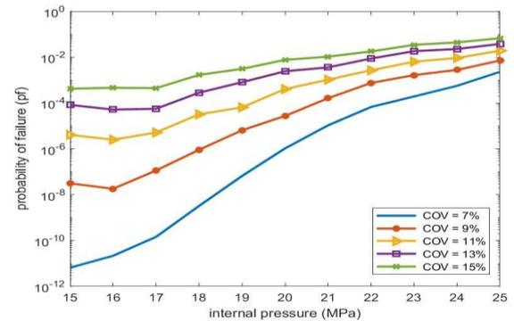
Fig. 7. Probability of failure in terms of the variation of the different COV of the hoop tensile strength
