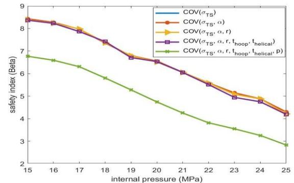
Fig. 6. Safety index under various considerations of input random design variables
