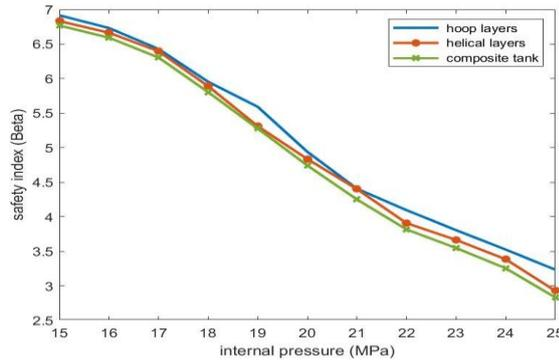
Fig. 4. Safety index of helical and hoop layers in terms of internal pressure
