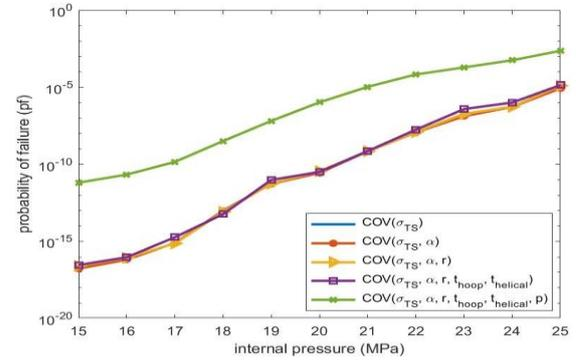
Fig. 5. Probability of failure under various considerations of random variables
