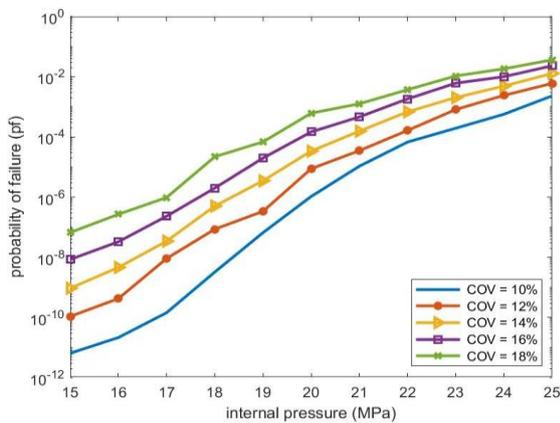
Fig. 9. Probability of failure in terms of COV of the internal pressure
