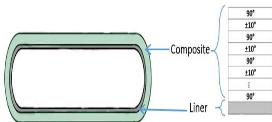
Fig. 2. A sketch of the composite tank and layer orientation
