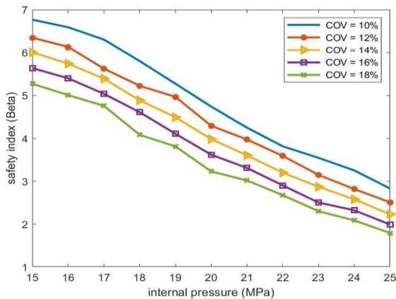
Fig. 10. Safety index in terms of the variation of the different COV of the internal pressure
