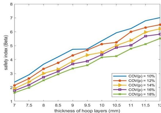
Fig. 18. Safety index of the hoop layers of the composite tank in terms of hoop thickness with the variation of different COV of the internal pressure (P=20MPa)
