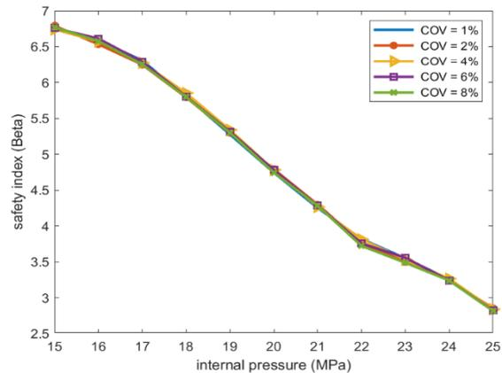
Fig. 12. Safety index in terms of different COV of the winding angle
