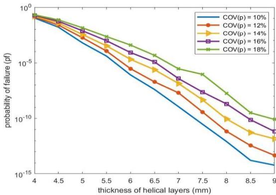
Fig. 15. Probability of failure of the helical layers of the composite tank in terms of helical thickness with the variation of different COV of the internal pressure (P=20MPa)
