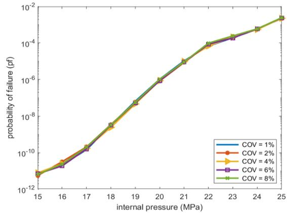
Fig. 11. Probability of failure in terms of different COV of the winding angle
