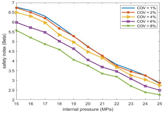
Fig. 14. Safety index in terms of the variation of different COV of the composite thickness
