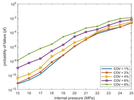
Fig. 13. Probability of failure in terms of the variation of different COV of the composite thickness
