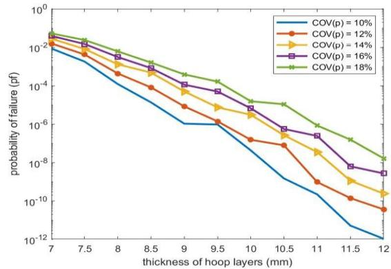
Fig. 17. Probability of failure of the hoop layers of the composite tank in terms of hoop thickness with the variation of different COV of the internal pressure (P=20MPa)
