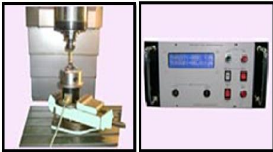
Fig.2. Drilling set-up with dynamometer and digital display
