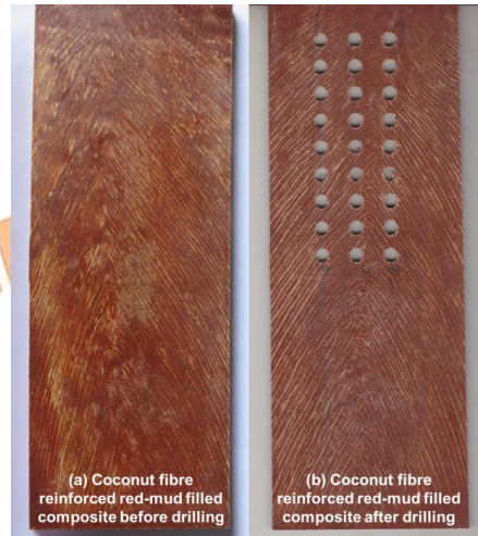
Fig. 1. Composite before and after drilling
