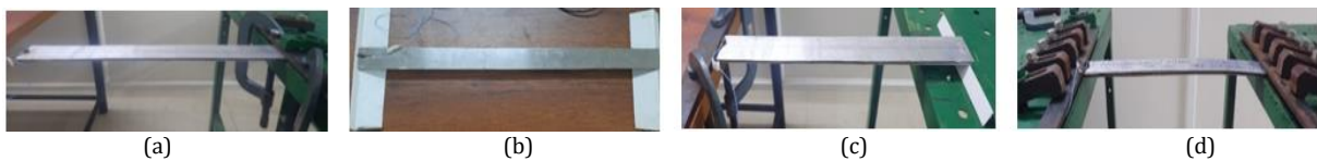
Fig. 7. Al - NR - SS viscoelastic sandwich beam under (a) C-F (b) S-S (c) C-S (d) C-C boundary conditions
