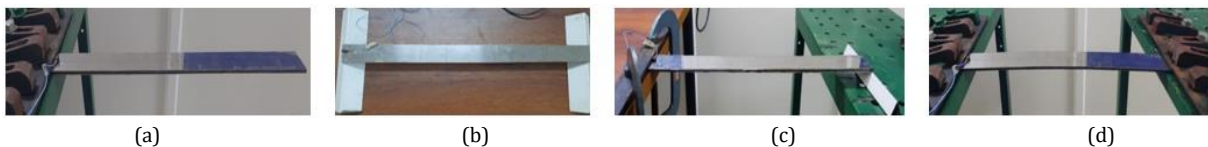
Fig. 8. SS - NR - SS viscoelastic sandwich beam under (a) C-F (b) S-S (c) C-S (d) C-C boundary conditions
