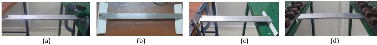
Fig. 6. Al - NR - Al viscoelastic sandwich beam under (a) C-F (b) S-S (c) C-S (d) C-C boundary conditions
