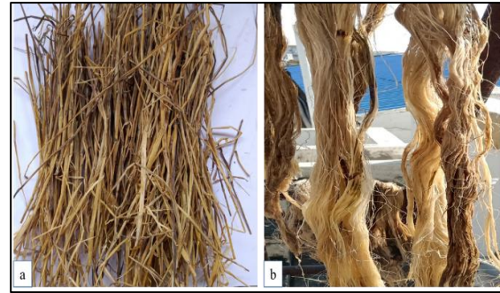
Fig. 1. Chemically treated fibers: (a) Paddy straw, (b) Pineapple leaf fiber
