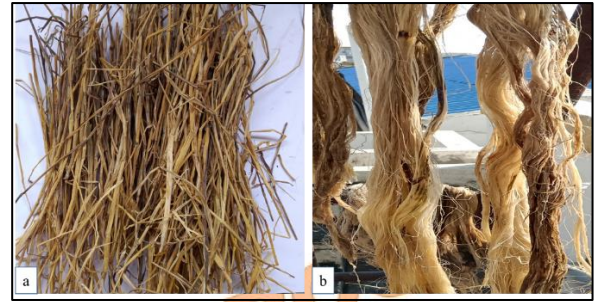
Fig. 1. Chemically treated fibers a) Paddy straw b) Pineapple leaf fiber
