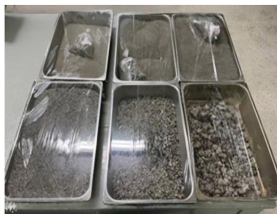
Fig. 3. Bottom ash (BA) that can be separated into different sizes
