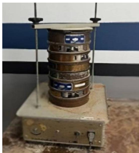
Fig. 2. Separation of bottom ash using a sieve
