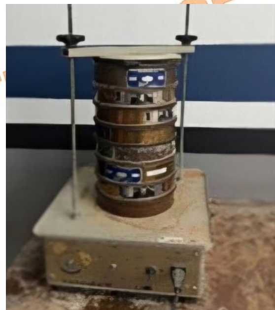
Fig. 2. Separation of bottom ash using a sieve
