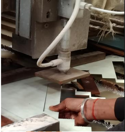
Fig. 3. a. Waterjet cutting off-axis (45°) Orientation
