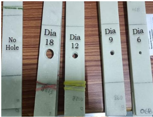
Fig. 3. b. Specimen with drilled holes
