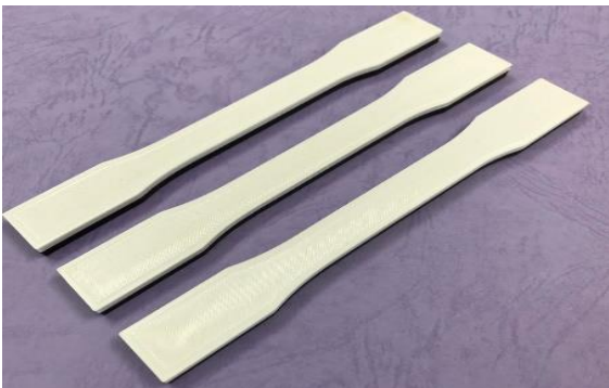
Fig. 4. Some of the test specimens printed with a 3D printer
