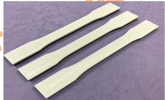
Fig. 4. Some of the test specimens printed with a 3D printer
