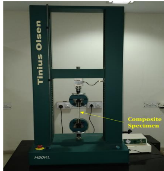
Fig. 4. Tensile testing of the composite specimen on UTM
