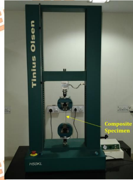
Fig. 4. Tensile testing of the composite specimen on UTM
