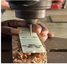
Fig 1: Specimen drilled for repair work.
