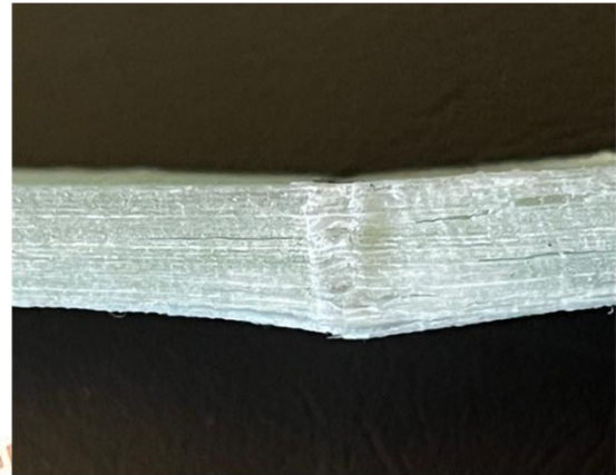
Fig 3: Delamination of glass fiber laminate after 3-3PBT
