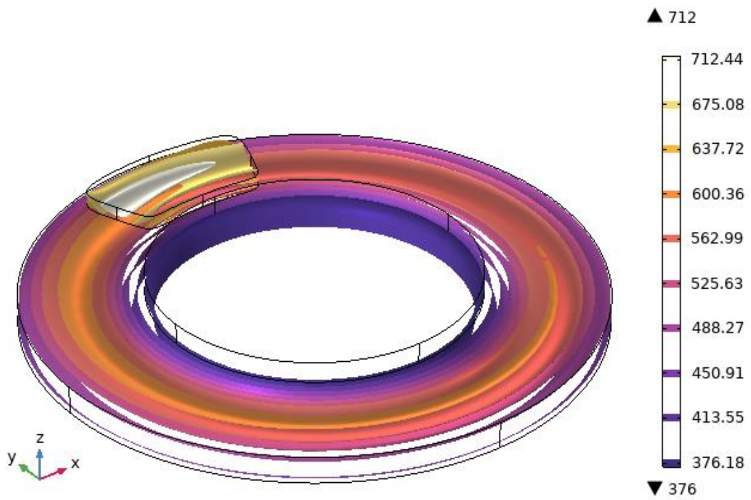
Figure 13. Isothermal contours of semi-metallic pad material
