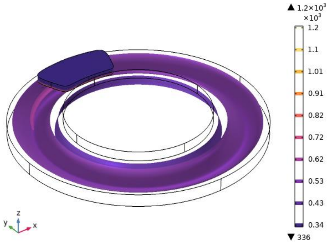
Figure 14. Isothermal contours of epoxy pad material
