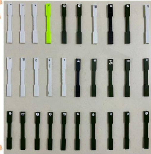
Fig. 5. Fabricated Additive Manufactured specimens [19]
