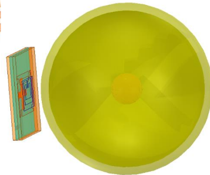
Fig. 10. Spherical breast phantom placed parallel to the designed antenna.
