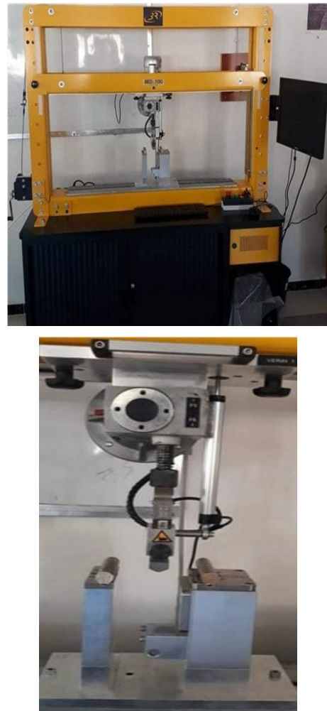
Fig. 3. Bending testing machine.
