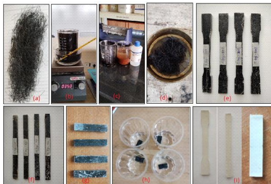
Fig. 3. Preparation of Treated Long Pig Hair fiber reinforced Epoxy Composite (a) Long Pig Hair, (b) Treatment with 0.25M NaOH, (c) Neutralized the fibers from Acetic Acid, (d) Drying process, (e) Tensile Test Samples, (f) Flexural Test Samples, (g) Impact Test Samples, (h) Water Absorption Test Samples, (i) Control Samples
